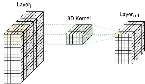
Fig. 3: A 3D convolution. In a 2D convolution, multiple 2D convolutional filters are stacked into a resulting 3D volume, whereas in a 3D convolution, 3D filters are stacked into a 4D volume, as show in Figure 4. The above graphic only represents one 3D filter.
