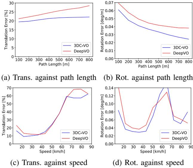
Fig. 6: Translation and rotation errors for 3DC-VO and DeepVO against path length and speed for the KITTI evaluation sequences 10-21.
