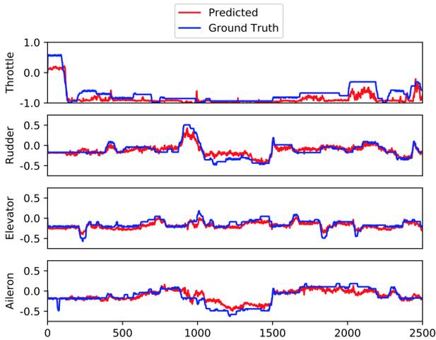
Fig. 7: Predicted (red) and ground truth (blue) joystick positions from a flight simulator sequence with a human pilot. Joystick axes have an affine relationship with thrust and angular velocity inputs. Offset from zero-mean is due to joystick calibration offset.
