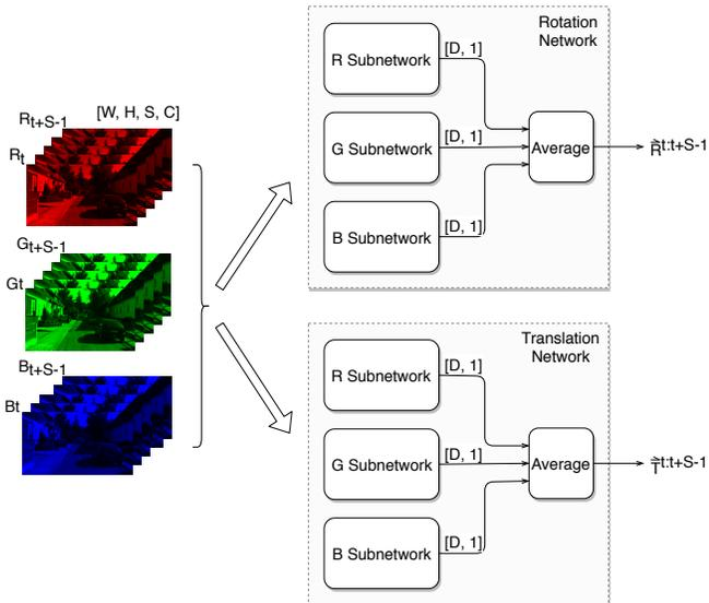
Fig. 2: High level 3DC-VO architecture. W, H, S, and C stand for width, height, stack size, and channels, respectively. D represents the number of dimensions of the output. For the KITTI task, each subnetwork outputs a single scalar, with the rotation network outputting the yaw offset between frame  $t$  and  $t + S - 1$ , and the translation network outputting the forward offset. For the quadrotor control estimation task, the rotation output is a three-dimensional angular velocity vector.
