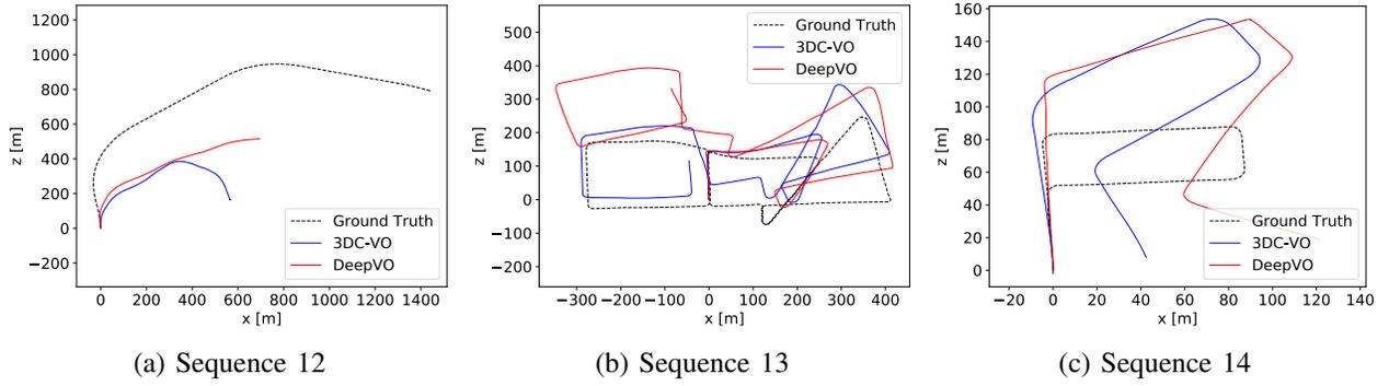
Fig. 5: Plots 12-14 of KITTI ground truth (in black), 3DC-VO predictions (in blue), and DeepVO predictions (in red). Although our method observes only a monocular image stream, making the odometry task susceptible to scale ambiguity, the scale of our estimated trajectories approximately match the ground truth.
