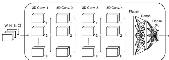
Fig. 4: Generic subnetwork structure. As with Figure 2,  $W, H, S, C,$  and  $F$  stand for width, height, stack size, channels, and number of filters, respectively, and  $D$  represents the network output dimension.
